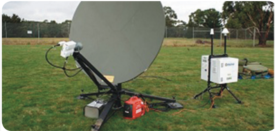
Satellite Cell on Wheels (SatCOW) showing 3G Mobile Base Station with Teledyne Paradise Datacom satellite modems
