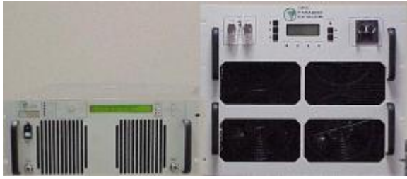
Figure 8. Comparison of new and old 400W, 6 GHz Solid State Power Amplifiers.
